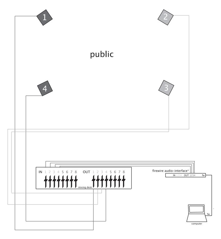
Cambuche - loudspeaker distribution \* computer and firewire interface can both be replaced by an ADAT player
